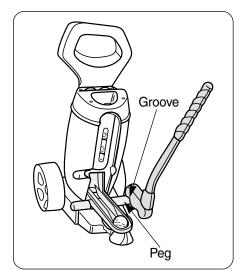
Fit one of the grooves on the driver or putter to the peg and push down.
